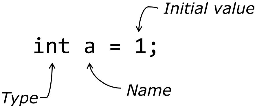
The diagram illustrates the components of the variable declaration "int a = 1;". It features three curved arrows pointing to specific parts of the code: one arrow points from the label "Type" to the word "int", another points from the label "Name" to the letter "a", and a third points from the label "Initial value" to the number "1".
